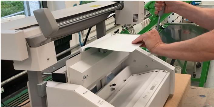
09. Pivot the clamp into position using the right-hand lever holding the cover back to expose the spine-edge.
