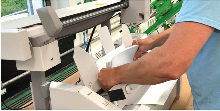
07. Carefully drop the printed pages down into the cover. First page facing the back and spine to the bottom.
