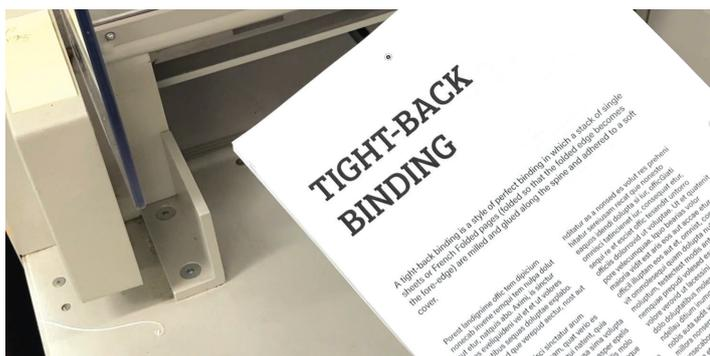
01. Stack and align the printed pages and trim the spine-edge to the crop marks to produce a flush edge.
