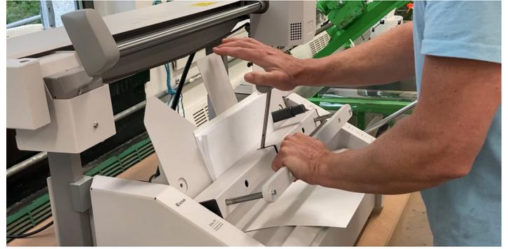
08. Push the clamp against the bookblock and lock in place by lifting the handle while holding the frame.
