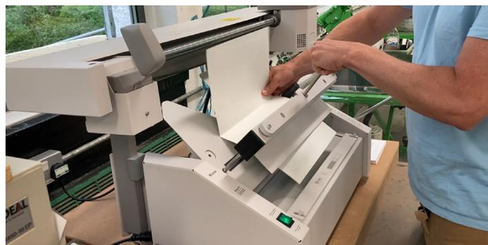
06. Raise the clamp and slide the cover in up against the stop with the front facing the back of the machine and the folded edge located snugly against the bottom.
