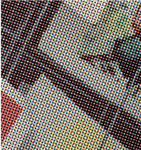
A close up example of a CMYK process print showing how the colours mix.
