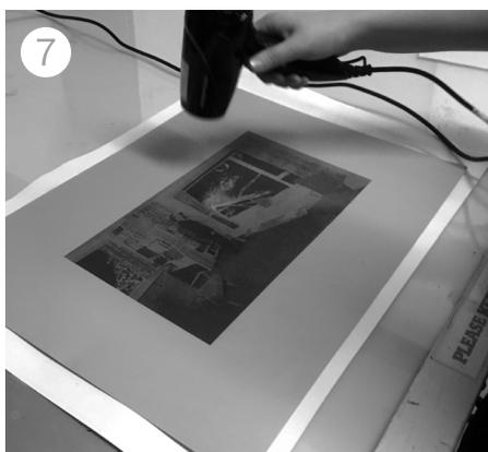
7 Dry the plate completely with a Hairdryer. Your plate is now ready for gumming.
