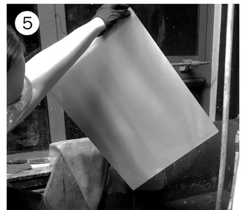
5 Lift the plate out of the tray and holding by a corner let the excess water drain off.
