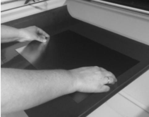
Carefully placing the photopolymer plate for the first exposure.
