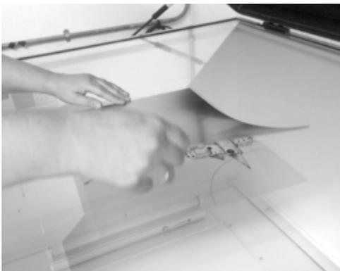
Placing the plate on the artwork for the 2nd exposure.
