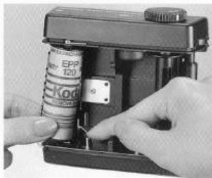
While holding down the left-hand Spool Release Pin of the Film Insert, fit a roll of film between the upper and lower left-hand Film Spool Studs. Make sure that the backing paper is set as shown in the photo above.
