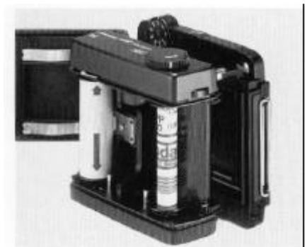
After correctly placing the insert into the housing, close the back cover, and while gently holding it in place, push both of the Back Cover Latches as far as they will go.
