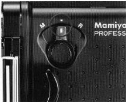
Before attempting to advance the film to the first frame, make sure the R-M Lever is set to its normal (center) position. If the lever is set to 'M'(multiple exposure), it will not be possible to advance the film with the Cocking Lever.
